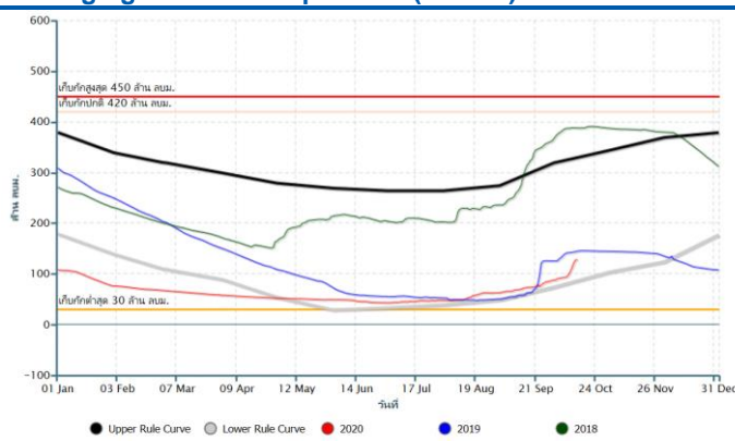
Figure 4: Khlong Si Yat dam in Chachoengsao postponed its surging time from September (normal) to October
